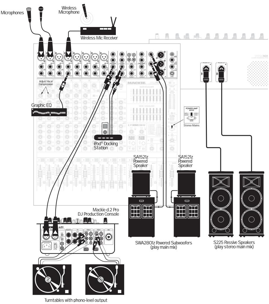
This diagram shows microphones connected to the mic inputs of channels 1 and 2, a wireless microphone receiver connected to the mic input of channel 4, and a graphic EQ connected to channel 4's insert jack (to help control any feedback in the wireless mic). An iPod docking station is attached to channels 11/12, using RCA to 1/4" TS adaptors.
